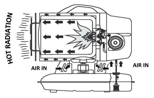
Airflow is necessary to ensure proper combustion, it is supplied by the internal burner fan. The air enters the burner funnel and gets mixed with a high-pressure fuel jet. The fuel flow is secured by an electrical pump, which sucks the fuel away from the tank and moves it to the nozzle under high pressure.
