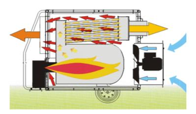
The unit is heating air that flows through it by combustion chamber and heat exchanger. Supply fuel is burnt in combustion chamber. Flue gas goes through heat exchanger outside to the chimney.
